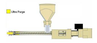
Empty the barrel of Ultra Purge and completely shut down the machine (turn off all heaters). <u>Do not</u> add any resin after Ultra Purge and don't leave the temperature idle
