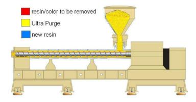
Adjust screw rotation to low to allow the compound to expand inside the machine.
