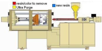
Keep the barrel of the press full of the resin/color you want to purge when adding the Ultra Purge to the machine (we recommend loading half of the barrel capacity of Ultra Purge for machines that are in good working condition) Step 3
