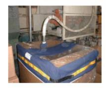
**IPS Gaylord Covers** By keeping your material securely covered within the container you prevent your raw material becoming contaminated with airborne dirt, dust, and other unwanted debris.
